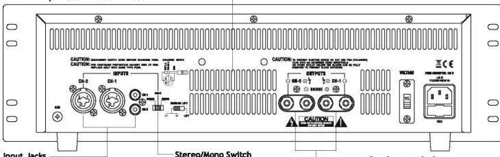
Input Jacks Let you connect a variety of audio input sources via the balanced (XLR/6.35mm phone jack combinations) or unbalanced (RCA) inputs.
